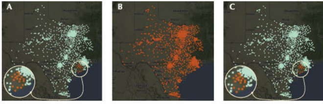
Fig. 4. Evaluation of the boundary defense mechanism. (A) The grid is under “zonal attack,” where the measurements within a zone are corrupted (shown in red). SE based on (B) Newton’s method for nonlinear least squares, and (C) the proposed method with SOC, where in both cases, buses with an estimation error greater than 0.002 are marked in red.
