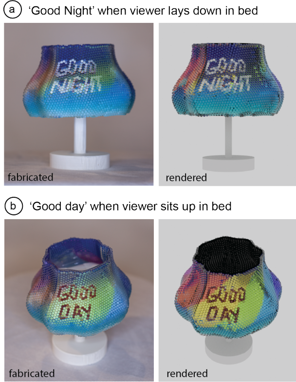
Figure 13: This lampshade displays different greeting messages when the users looks at it from different heights (laying down in bed vs. sitting up in bed).
