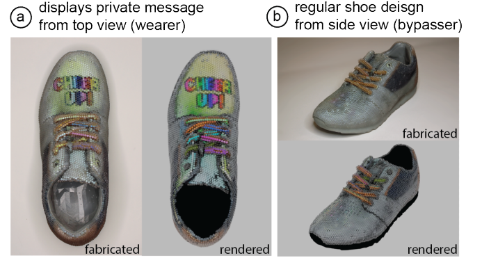
Figure 15: Visual designs only visible from the user's viewing angle: (a) A pair of shoes that shows a supportive message to the wearer looking down on the shoes, which (b) other people looking from the side at the shoes cannot see.
