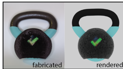
Figure 1: 3D printed objects with lenticular lens surfaces enable viewers to see different appearances from different viewpoints (a: looking down; b: looking horizontally; c: looking up). Our user interface supports designers in setting up different viewpoints and assigning the corresponding textures. On export, it automatically generates the files for fabrication. Designers can then 3D print the object geometry, lenses, and underlying color patterns in a single pass with a multi-material 3D printer.
