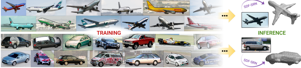
Figure 1: Learning 3D SDF shape reconstruction from static images. SDF-SRN learns implicit shape reconstruction from single-view images and 2D silhouettes at training time, allowing practical applications of real-world 3D object reconstruction trained from static image datasets.
