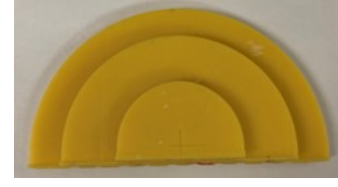
Fig. 1. Thin walls with half-cylindrical shapes printed in an SLA process
