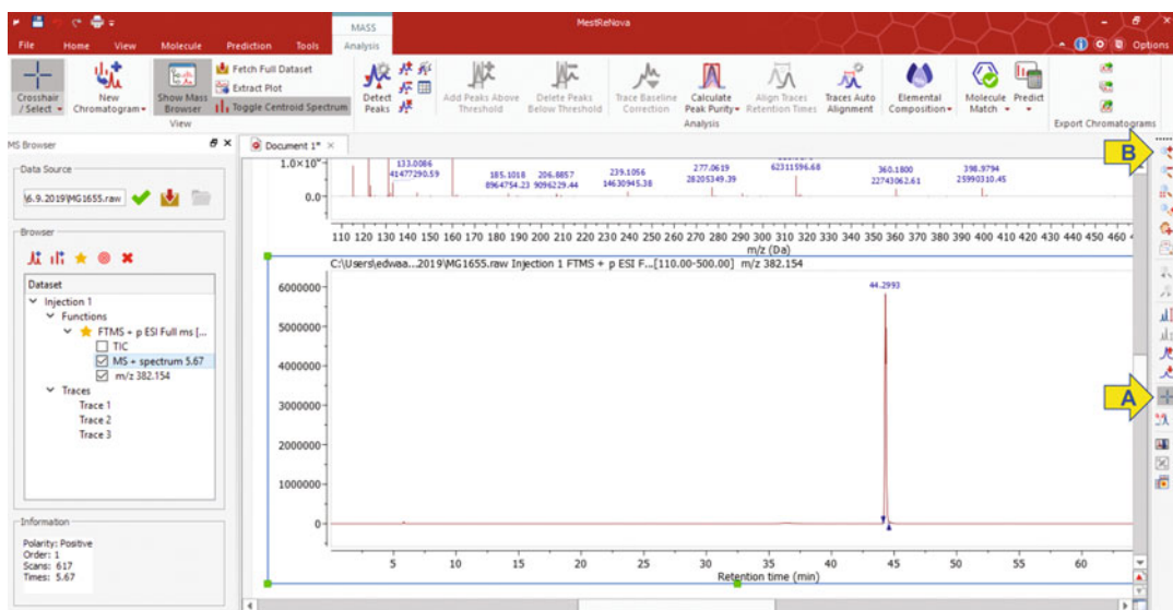
Fig. 4 Extracted ion chromatogram of 382.1544 m/z and the corresponding retention times of all analytes that fall within 5 PPM of this m/z of interest. Arrows indicate commands for selecting the range (a) and zoom in (b)
