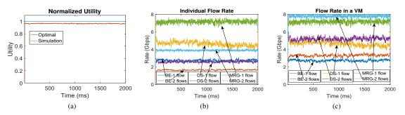
Figure 3: Normalized utility and rate allocation for half hosts having one flow and half hosts having two flows : (a) Normalized utility; (b) Average flow rate; and (c) Total per VM rate.
