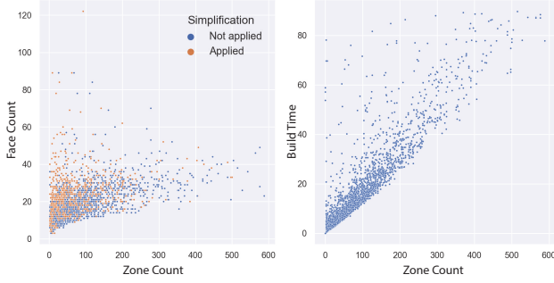
Figure 3: Zone graph construction statistics. (Left) Zone count vs. B-rep face count. (Right) Zone count vs. zone graph construction time (in seconds).
