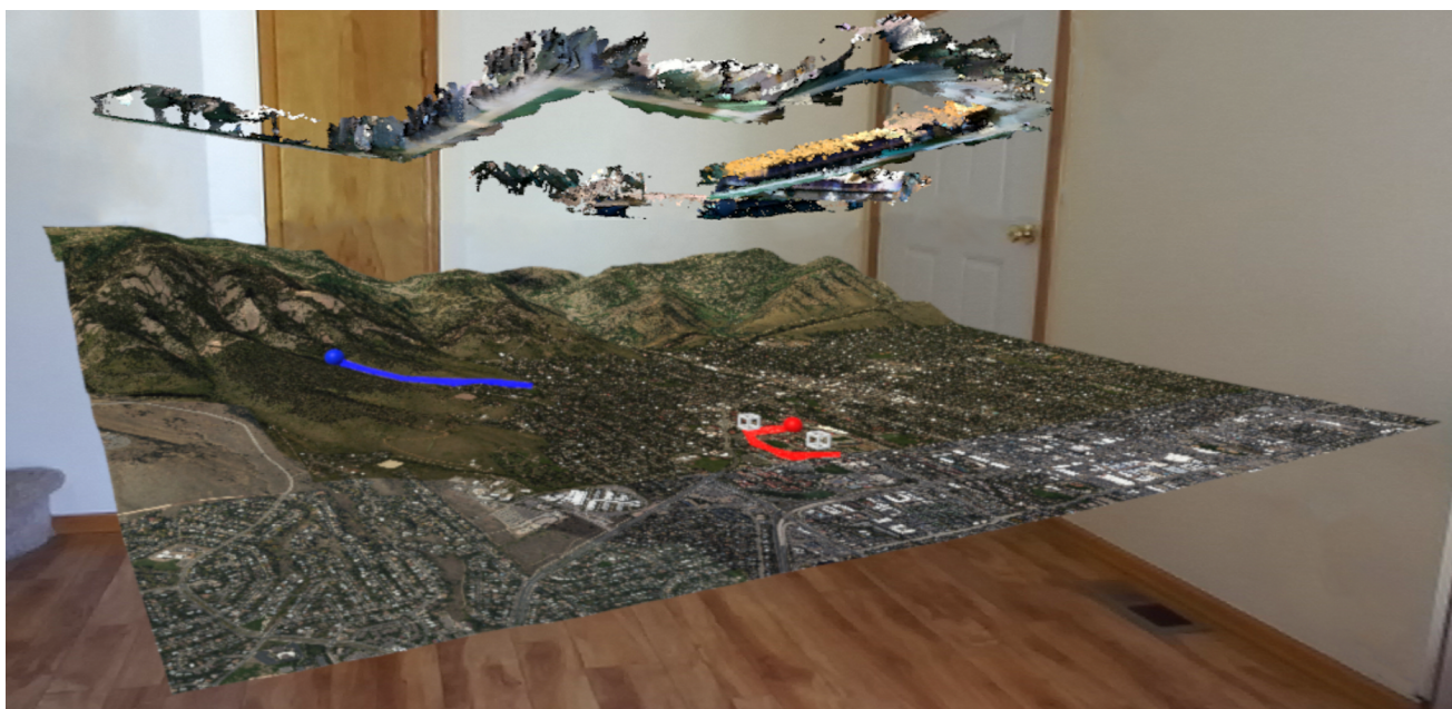
Figure 1: Mixed reality 3D terrain of field teams’ operating area seen from a video pass-through HMD. Current position and previous trajectory of human team (blue) and robot (red) are rendered contextually on the table. Above the terrain table, a dense RGB point cloud can be manipulated (position, rotation, scale) with the user’s hands.
