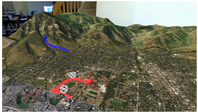
Figure 2: Trajectories (lines) and current GPS positions (spheres) of the human field team (blue) and the field robot (red). White cubes represent robot-collected 3D reconstructions that users can select to view and manipulate the corresponding MR dense point clouds above the 3D terrain table.
