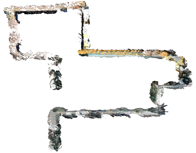
Figure 6: Large-scale 3D reconstruction of the robot’s path through a remote outdoor environment. See Figure 7 for a closer view of the reconstruction from the user’s perspective.
