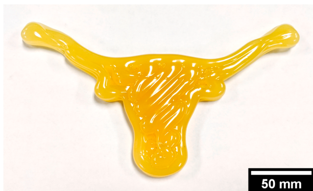
Fig. 7. Longhorn created in 3 min via reactive extrusion additive manufacturing. The part is 230 mm from horn tip to horn tip, 95 mm from the top of the head to the end of the snout, and 16 mm thick.
