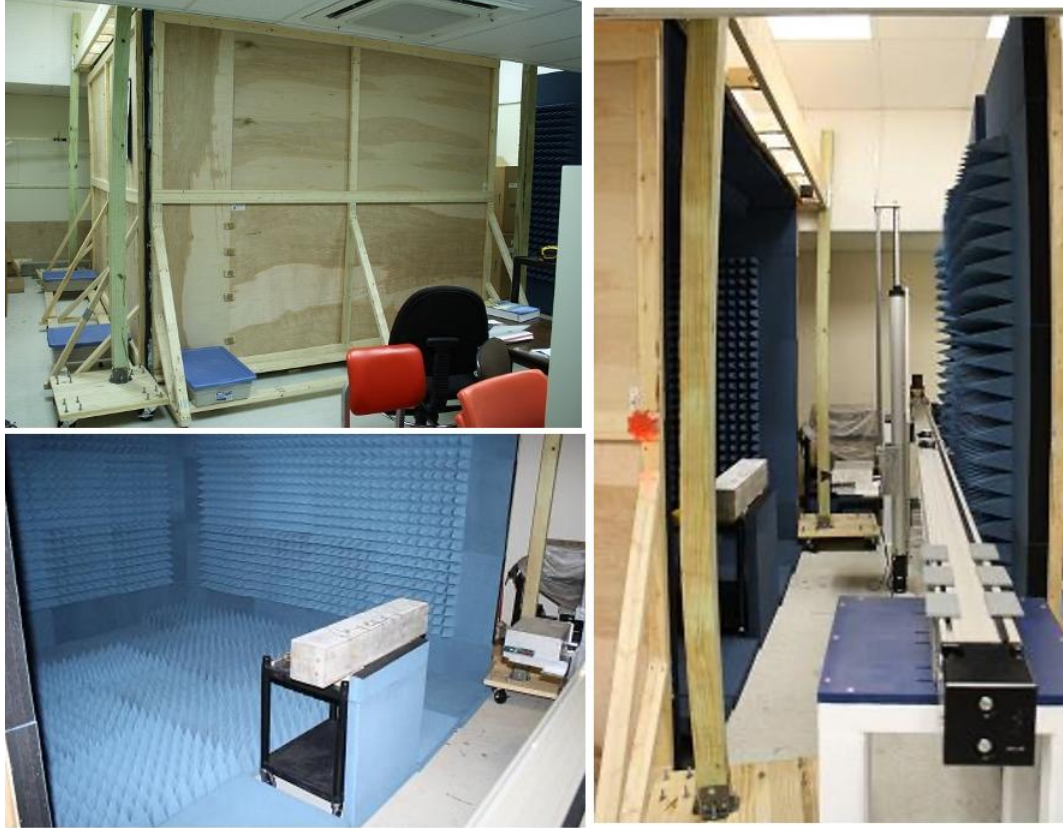
Figure 5. Exterior of the anechoic chamber for laboratory SAR imaging
