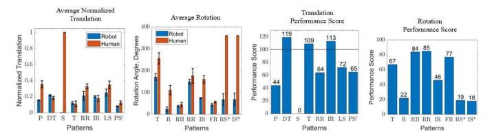
Fig. 4. Quantitative results from benchmark testing. Error bars represent one standard deviation from the mean. Patterns marked with an asterisk (\*) are evaluated as incomplete. Patterns marked with a dagger (†) are evaluated as non-anthropomorphic. For performance scores, a score of 100 indicates equivalence between the robot and human.
