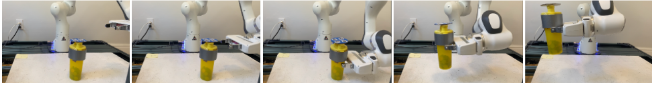
Fig. 4. Sequence of images showing the Franka robot arm performing a dynamic pickup task using our learned reactive and predictive controller. The controller generalizes to previously unseen locations of the object and performs the task with 80% success rate.
