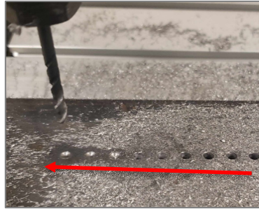
Figure 9: Drilling bit deterioration after drilling multiple holes
