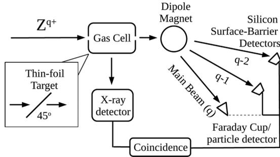
FIG. 2. Schematic diagram of the experimental setup. For the gas targets the setup is that shown in the main part of the figure with gas cell placed in the beam line. To measure the thin-foil targets, the gas cell is removed and the setup shown as the inset in the lower left of the figure is installed in the beam line.
