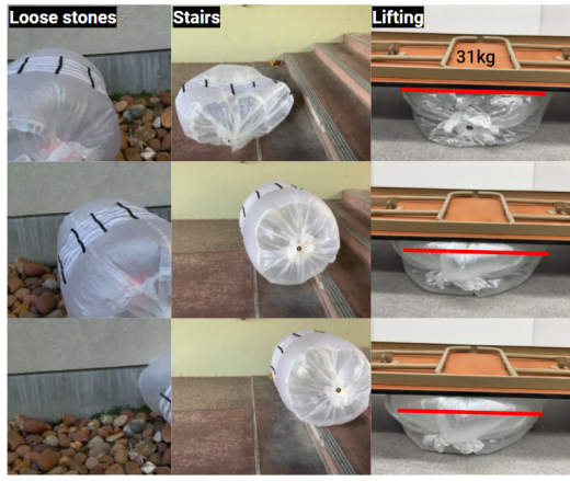
Fig. 10. Left: From top to bottom, an inflated SPHR navigates smoothly across loose rocks. Middle: Reaching an obstacle, the robot is able to inflate and climb an obstacle 12 cm in height. Right: After driving deflated to crawl under an obstacle, the robot is able to inflate and lift the object.
