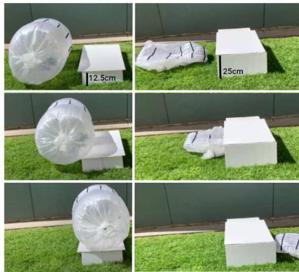
Fig. 1. The soft pneumatic hybrid robot (SPHR). Left : The robot is capable of rolling to an obstacle and climbing over it when fully inflated. Right : When approaching an obstacle deflated, the robot can pass underneath it.
