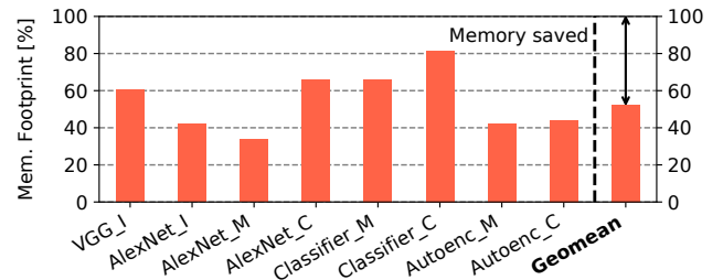
Figure 7. CODE Ensembles memory footprint with respect to baseline for the entries of Table 1.
