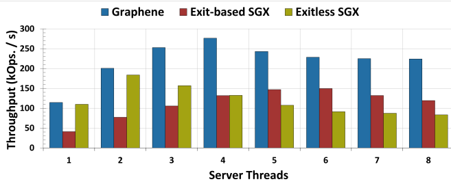
Fig. 3: Memcached performance measured in operations per second for a variable number of server threads. 4 clients are served concurrently.
