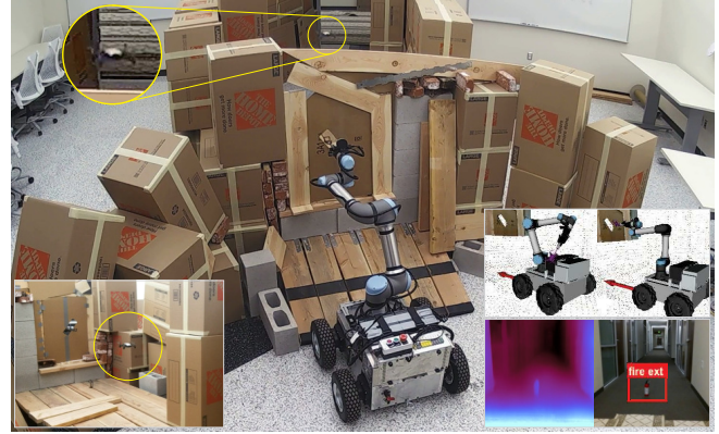
Fig. 1. Autonomous heterogeneous robotic system exploration into a partially-collapsed setting, by detecting aperture -like ingress points, inserting two micro-sized MAV scouts, and conducting visually-servoed exploration through remote guidance by the MMS. Corresponding video available at: https://www.youtube.com/watch?v=Avt0Gnv3CAI
