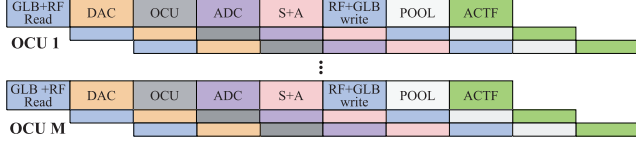
Fig. 5: The optical convolution unit pipeline.
