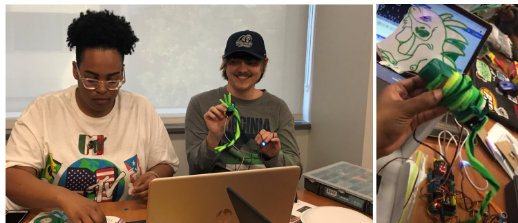
Figure 1: Preservice teacher, Briana, and engineering student, Craig, collaborated to design, build, and code a robotic chameleon prior to planning their lesson for Keith. Cerberus’ tail wags when petted (activated via distance sensor) and eyes light up when spoken to (activated via sound sensor).
