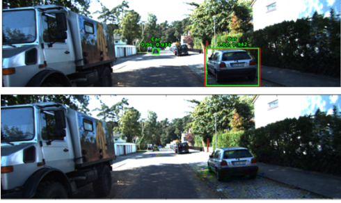
Fig. 1. Results of some of our disappearance attacks. Top is benign images and bottom is adversarial images. The 1st value corresponds to the classification confidence and the 2nd value corresponds to the IOU with the ground truth bounding box. The red boxes are ground truth and the green boxes are bounding boxes outputted by the model.
