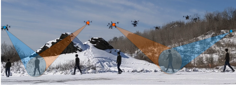
Fig. 1: We present a multi-UAV system for 3D human reconstruction in the wild. Our framework coordinates the motion of multiple aerial cameras to optimally reconstruct the dynamic target’s 3D body pose while avoiding obstacles and occlusions. We deploy the system in challenging real-world conditions and target motions such as jogging and playing soccer.
