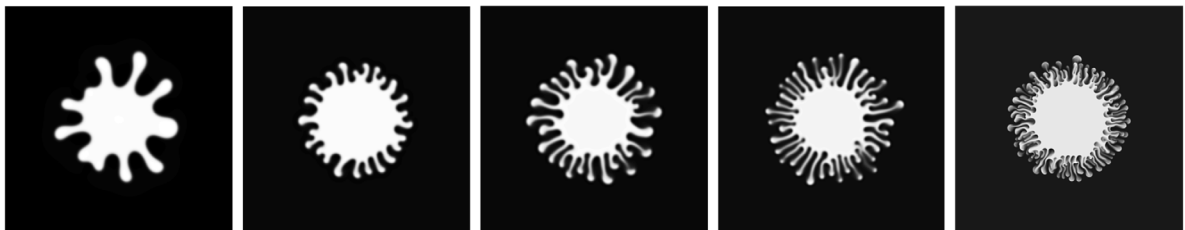
Fig. 4.12. Comparison of number of fingers where \lambda = 0.01, 0.001, 0.0005, 0.0001 , and 0.00001 , from left to right.
