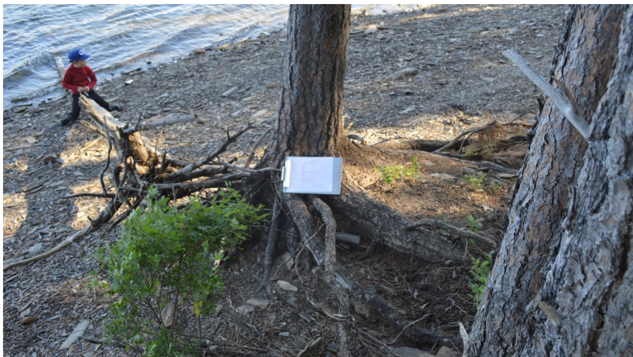
Figure 10. Specimen "E", typical of root structures that did not stabilize the bank. Note that erosion occurred on 80% of the base of the tree. This specimen had a deep taproot but had very few of the spreading woody roots or sinkers. Interlock only in the area not eroded.
