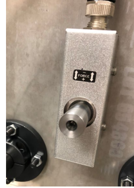
Figure 2: Load cell to measure web tension
