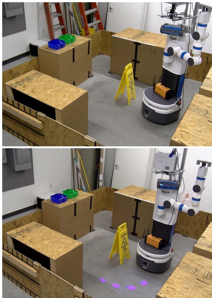
Fig. 1. A Fetch mobile manipulator navigating around a wet floor sign without (upper) and with (lower) arrow projection (purple). Despite of the effectiveness of arrow projection for revealing navigation path, no public code is readily available. Here we share such code in ROS and provide hardware support. Additional videos are available in [13], [14].
