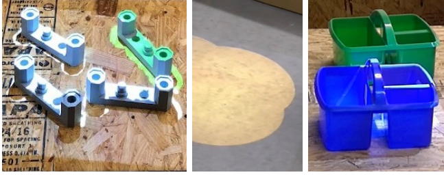
Fig. 3. Three other visualizations to show the generalizability for our work: point cloud for perceived objects [58], multiple spheres for ground obstacle, cube for caddy section. Any rviz visualization can be projected.
