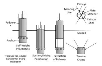
Fig. 1. The installation procedure of the MRA [5]
