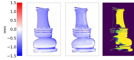
Figure 10: Results of our denoising model on a depth map from the physical scanner. The model was trained on synthetic data. From left to right: Depth errors after reconstruction, after denoising, improved regions.
