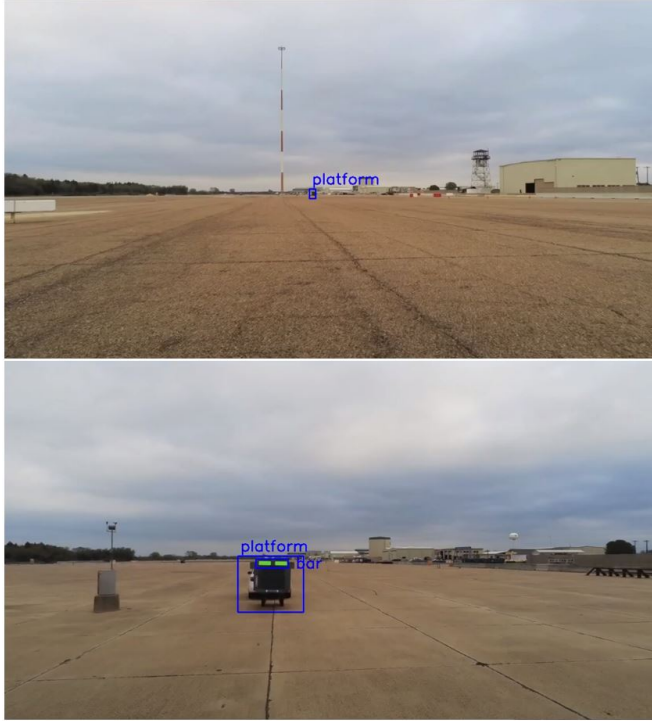
Figure 4. Long and mid-range real-time object detection result
