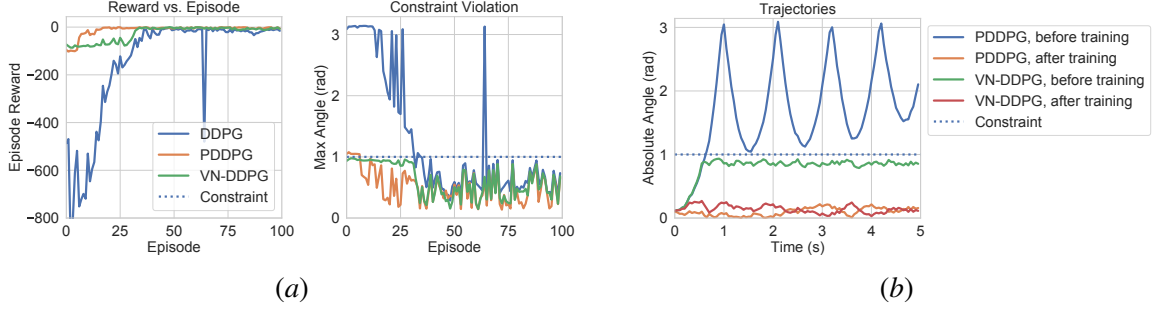
Figure 3: (a) Comparison of accumulated reward and constraint violation (max angle) for the pendulum problem. (b) Representative trajectories (angle vs. time) generated by the policy before training and after training.
