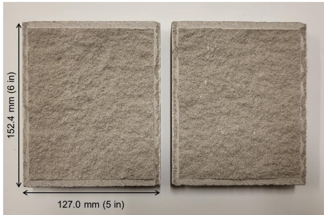
Fig. 1. Indiana limestone joint specimen with a tensile-fractured rough surface.
