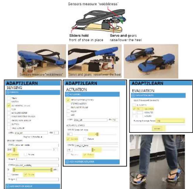
Figure 9: Adaptive heels that support learners in training to walk in high heels. Configuring the learning algorithm for the adaptive heels using Adapt2Learn 's user interface to set four synchronized ultrasonic distance sensors (two per shoe), and two synchronized servo motors.
