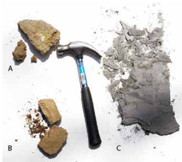
FIGURE 4: Examples of rock fragments produced from striking hand samples with the rock hammer. A: limestone breaks cleanly into large chunks. B: sandstone breaks into sand-sized grains. C: shale breaks into clay-sized particles and thin rock layers.
