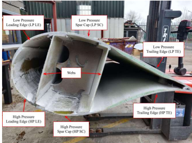
Figure 3. Cross section of LM 13.4 blade at maximum chord (2.51m from root end), with naming convention labels.
