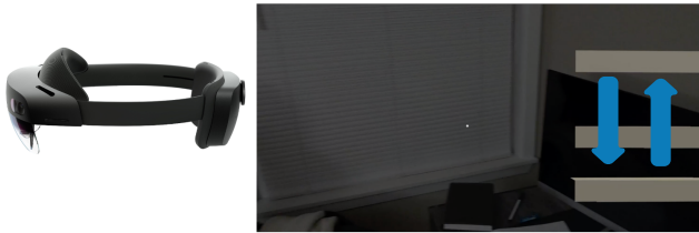
Figure 1: The design of our AR-based gait metronome running on Microsoft HoloLens 2 headsets.
