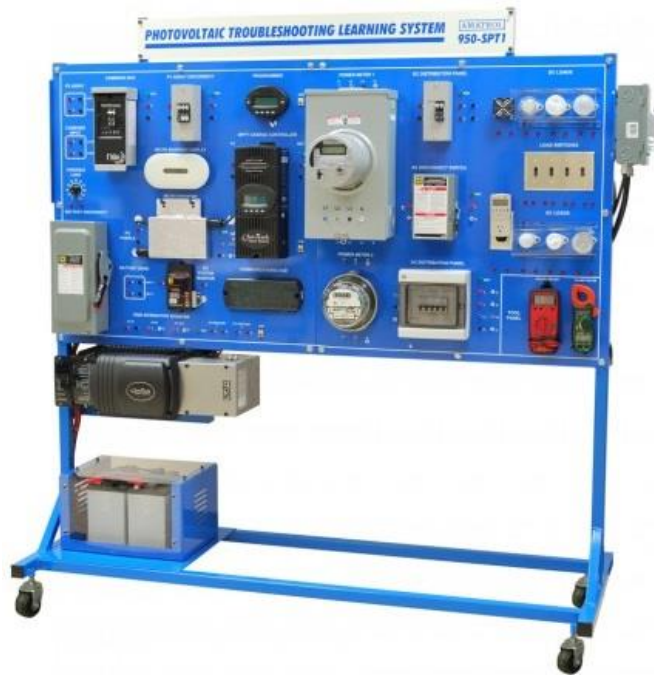
Fig 5. Solar PV Troubleshooting [9].
