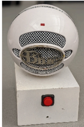
Fig. 1: Recording device that integrates a Raspberry Pi, Blue Snowball USB microphone, and a real-time clock.
