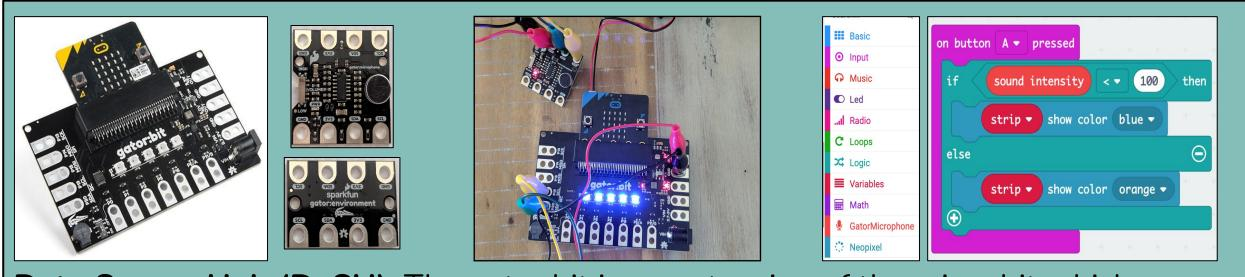
**Data Sensor Hub (DaSH)**: The gator:bit is an extension of the micro:bit which exposes more pins for alligator clippable sensors that measure temperature, soil moisture, sound, humidity,  $CO_2$ , etc. It provides functionality for simple data displays using LEDs and a speaker. Students program the micro:bit using MakeCode.
