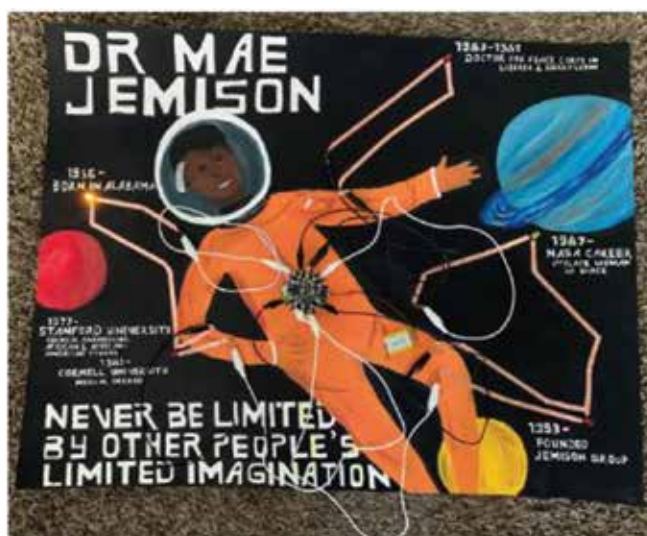
FIGURE 1: Left: circuitry diagram clearly distinguishing between positive and negative lines. Right: completed Mae Jamison timeline with the LEDs programmed to light up in sequence.
