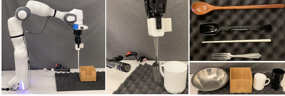
Figure 4: Physical setup and tools for robotic impact dataset collection. (Left) A Franka Panda holds and rotates a ceramic chopstick to swing at the wood napkin holder, with audio recorded by the bottom-left microphone. (Middle) Close up of a fork swung at a mug, with microphone at left. Objects were rested on a soft foam pad to prevent sliding and mitigate contact damping and acoustic reflection from the hard tabletop. (Right top) The tools used for striking (from top): wooden spoon, polycarbonate spoon, ceramic chopstick, and steel fork. (Right bottom) The struck objects (from left): steel bowl, wood napkin holder, ceramic mug, and polycarbonate cup.
