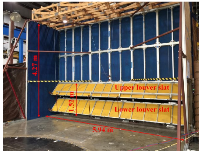
Figure 1 Downburst simulator at WOW with the two louver slats opened at 45^\circ
