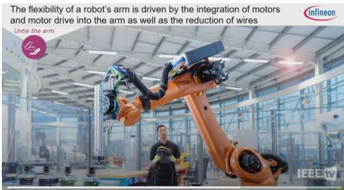
Figure 90: Industrial robot arm with external cabling, drive, and motor (source: Infineon).
