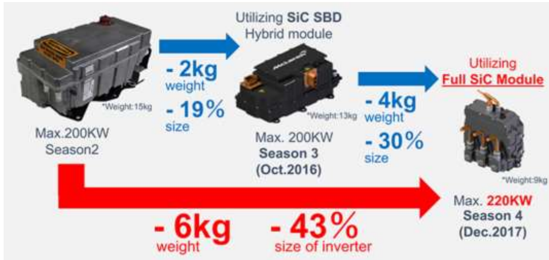
Figure 2: Inverter size and weight reduction (source: ROHM Semiconductor).
