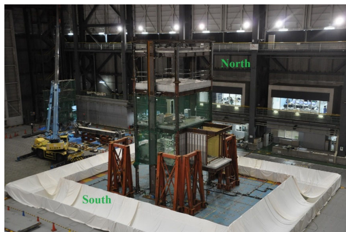
Fig. 1 – Test building on shake table
