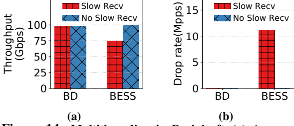
Figure 14: Multithreading in Backdraft, (a) Aggregate throughput, (b) Drop rate of victim flow. Backdraft achieves 100 Gbps using multiple cores while ensuring zero drop at the vswitch. In this experiment, applications are allocated enough number of cores to drive 100 Gbps.
