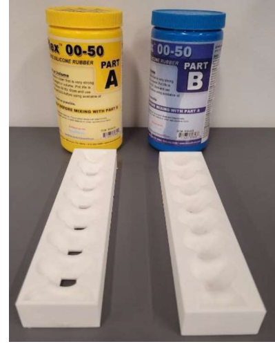
Fig 4: Top (left) and bottom (right) part of the mold and silicone used (Ecoflex 00-50)
