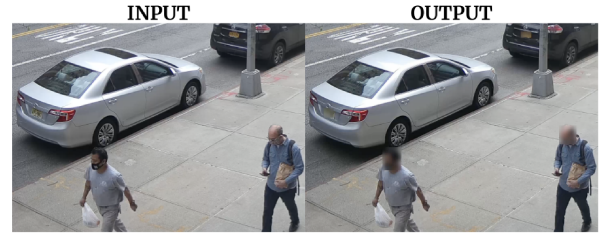
Fig. 7: Input (left) and output (right) of the face and license plate blurring pipeline.
