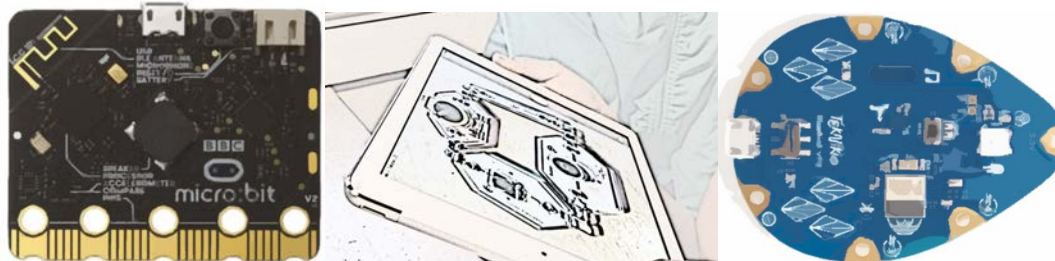
Figure 2: On the back of the Micro:Bit, components, such as the processor and BLE antennae, are labeled [37]; A LightUp AR tablet app makes circuit concepts visible to learners [31]; the shape of the Bluebird microcontroller evokes new communities and possibilities [17].
