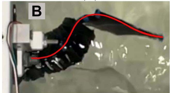
Fig. 5. (A) Tracked shape of  $38.71 \text{ cm}^2$  triangle tail for one swimming cycle (0.834 seconds) under the assumption of constant curvature. The color (ROYGBV) corresponds to the chronological progression of the tail.  $t = 0 \text{ s}$  corresponds to red and  $t = 0.834 \text{ s}$  corresponds to violet. (B) A snapshot of the physical model during the same locomotion experiment with a curve (red) overlaid to indicate the tracked shape. Snapshot taken at  $t = 0.004 \text{ s}$ .
