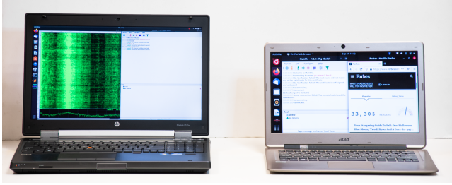
Figure 1: Experimental setup example. Attacker laptop (left) and victim laptop (Acer Aspire S3, right). Attacker and victim are both connected, via WiFi, to a Mumble VoIP chat room session. The green spectrogram on the attacker conveys the audio stream received from the victim.
