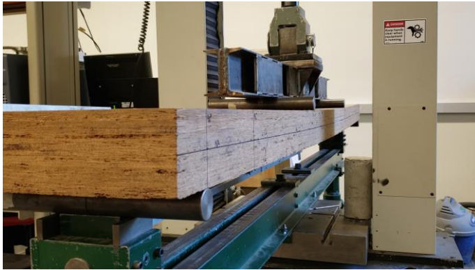
Four-point-bending l/d \geq 20
