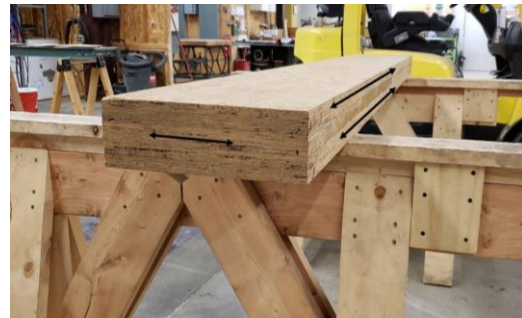
Cross laminated strand veneer lumber (CLSVL) – mass timber product
