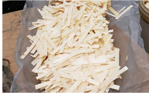
Wood strands ready for thermal modification
